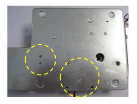
3- Reverse the boltwork, and then locate and remove the 2 retaining screws of the defective switch
