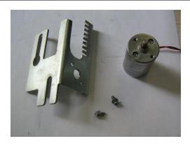
6- Separate the motor from the bracket
