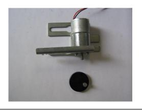
4- Remove the cam from the motor
